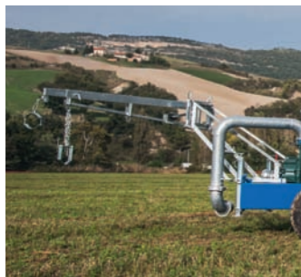
Arm-holder to lift up the suction pipe
