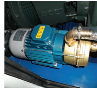
Electric priming vacuum pump
