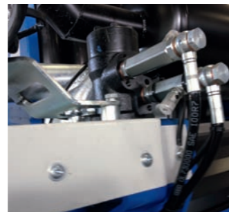
Self-braking system for arm
