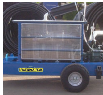
Engine roof + net-guard
